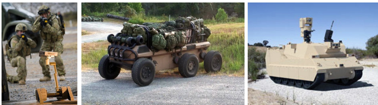
Fig. 10 The SUGV, MULE, and ARV are the ground vehicles defined by the Army's Future Combat Systems program.
